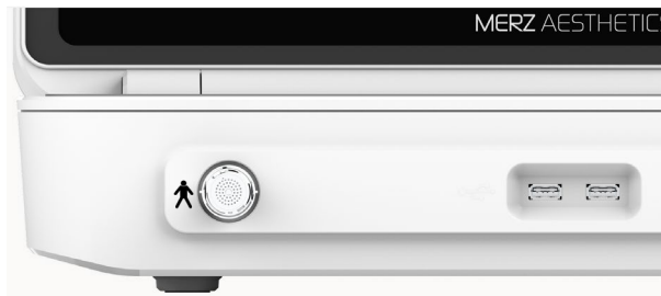
Figure 5.1 Handpiece Connector Receptacle.
